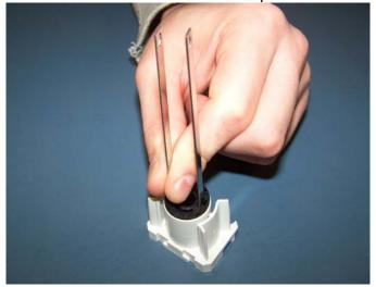
**11.** Replace clutch cover by snapping it into place.
