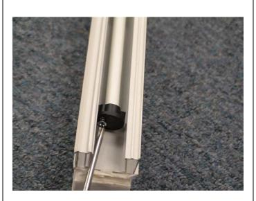
**10.** If the new continuous loop has not been placed into the clutch, you will need to wrap the new loop around the teeth until the loop is completely wrapped around the clutch.
