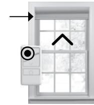
2. Press and hold the UP and DOWN buttons at the same time for 3 seconds. When the remote LED turns amber, release both buttons.
